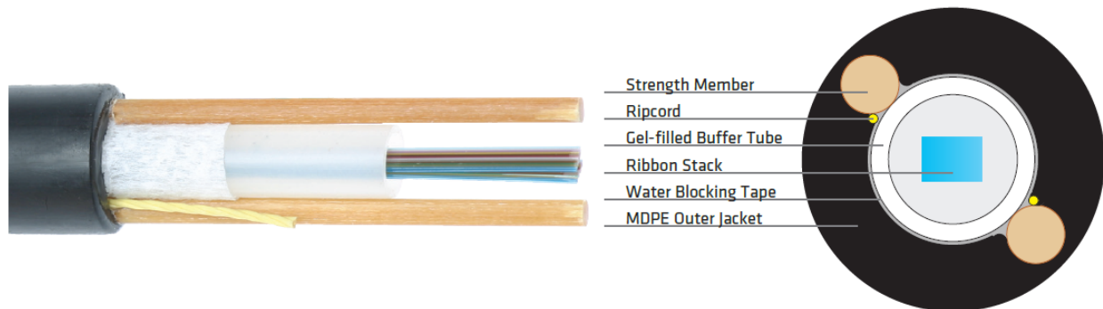
Figure 3: Cross sectional view of the multicore fibre optic cable used for the evaluation
