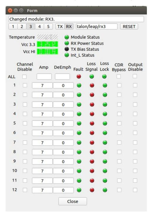
The internal GUI working prevent out of range values from being written to the device by validating all input prior to action. If an input value is out of range, the previous value is replaced, and the user is informed that the value is out of range via the status display at the top of the window.
